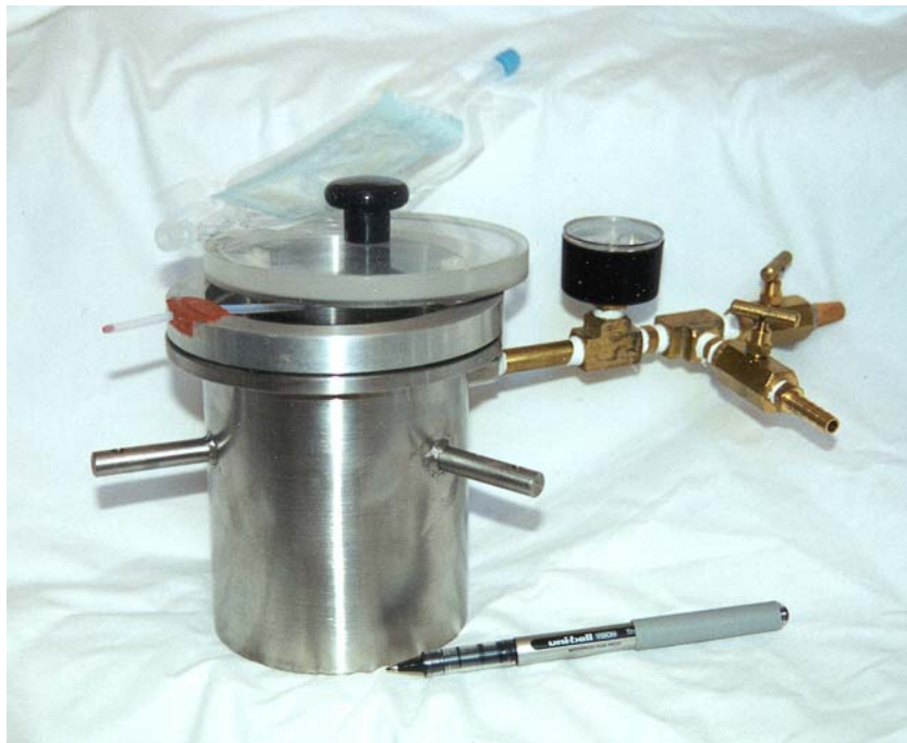
Figure 2. Vacuum Chamber and Plasma Processing Bag
