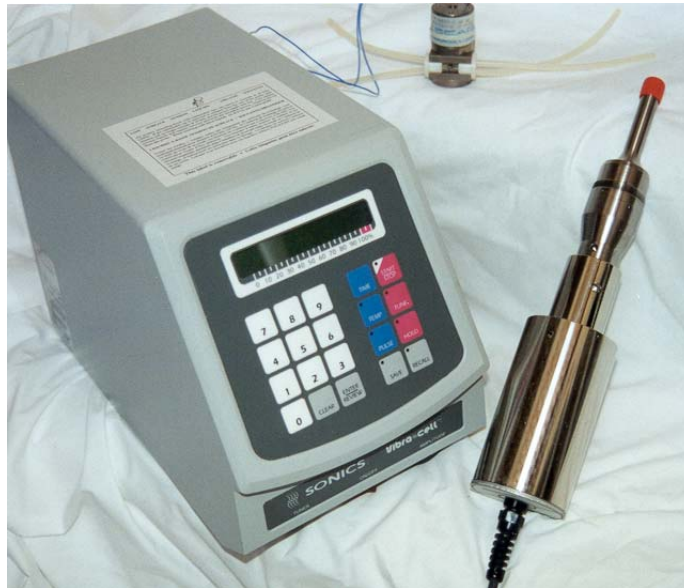
Figure 5. Ultrasonic Driver for Ozone Mixing Nozzle
